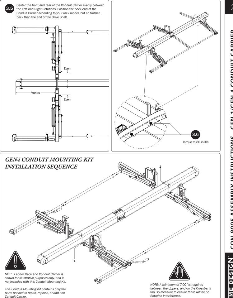
CON-8005 ASSEMBLY INSTRUCTIONS- GEN 1/GEN 4 CONDUIT CARRIER
