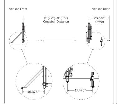
6.00 Ft: Drill holes into the Service Body mounting location according to dimensions shown.
