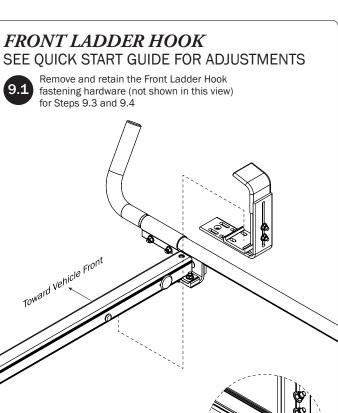
Seat the Front Ladder Hook into the lower Crossbar groove as shown in this bottom view
