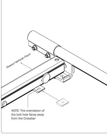
Place the Clamp Bracket removed in Step 0.2 into the lower groove of the Crossbar, and slide it on top of the Front Clamp Down Tube Holder
